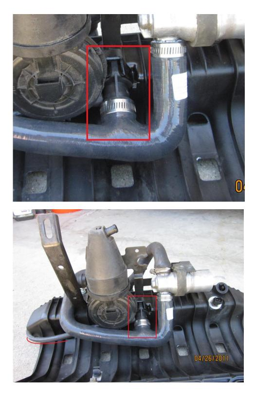
**#2 – Throttle Body Seal** – The problem is a M50 manifold has a seal gland for a seal to be installed into. The M52 throttle body also has this gland for the seal to be installed into. Photo right.
